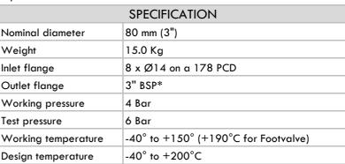
NB: temperature range vary according to o'ring material
