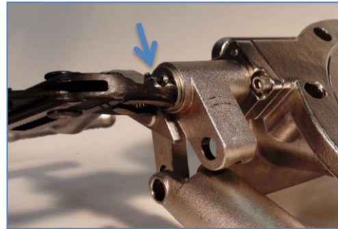
7 - Remove the split pin of the drive yoke
