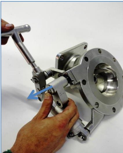
8 - Remove the drive yoke
