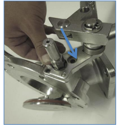
14 - Put the stuffing clamp & the handle
